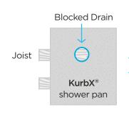
Use an **ExtendIT Mini Pitch Filler** to move drain away from joist
